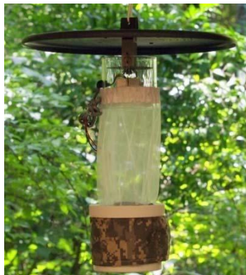
Figure 1.3.2: CDC Light Trap. Miniature Light Trap Model 512 (John W. Hock Company) http://johnwhock.com/products/mosquito-sandfly-traps/cdc-miniature-light-trap/
