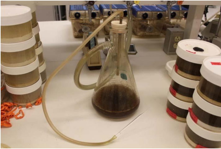
Figure 4.3.2. Vacuum aspirator with soapy water in the bottom for aspiration sand flies from oviposition pots.
