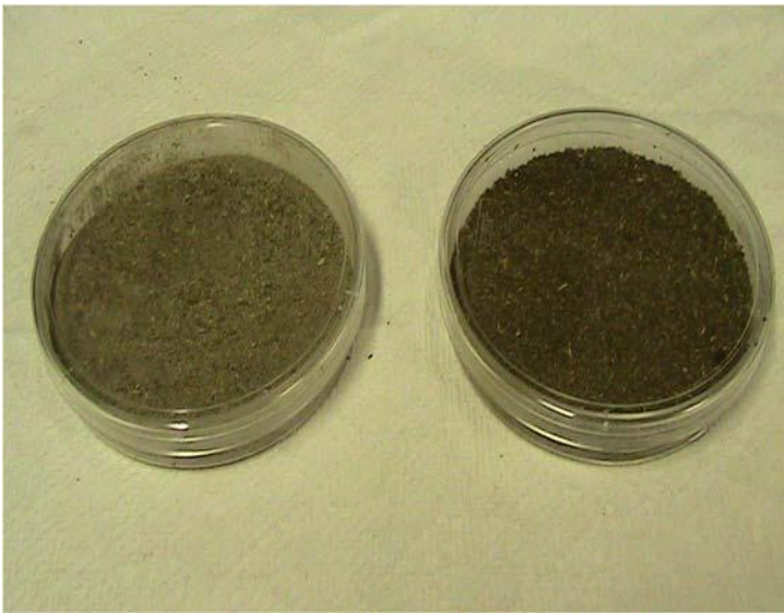
Figure 4.7.1. Dish on the left containing a grey/light brown powder (bad) and dish on the right containing a dark brown powder (good)
